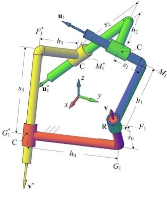
Non-italic R and C represent R joint and C joint respectively
