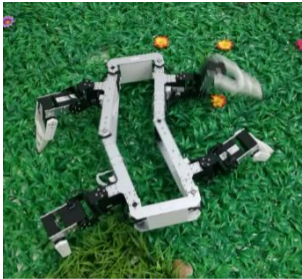
(b) Step 3: body twists back and leg 2 in transfer referring to figure 4
