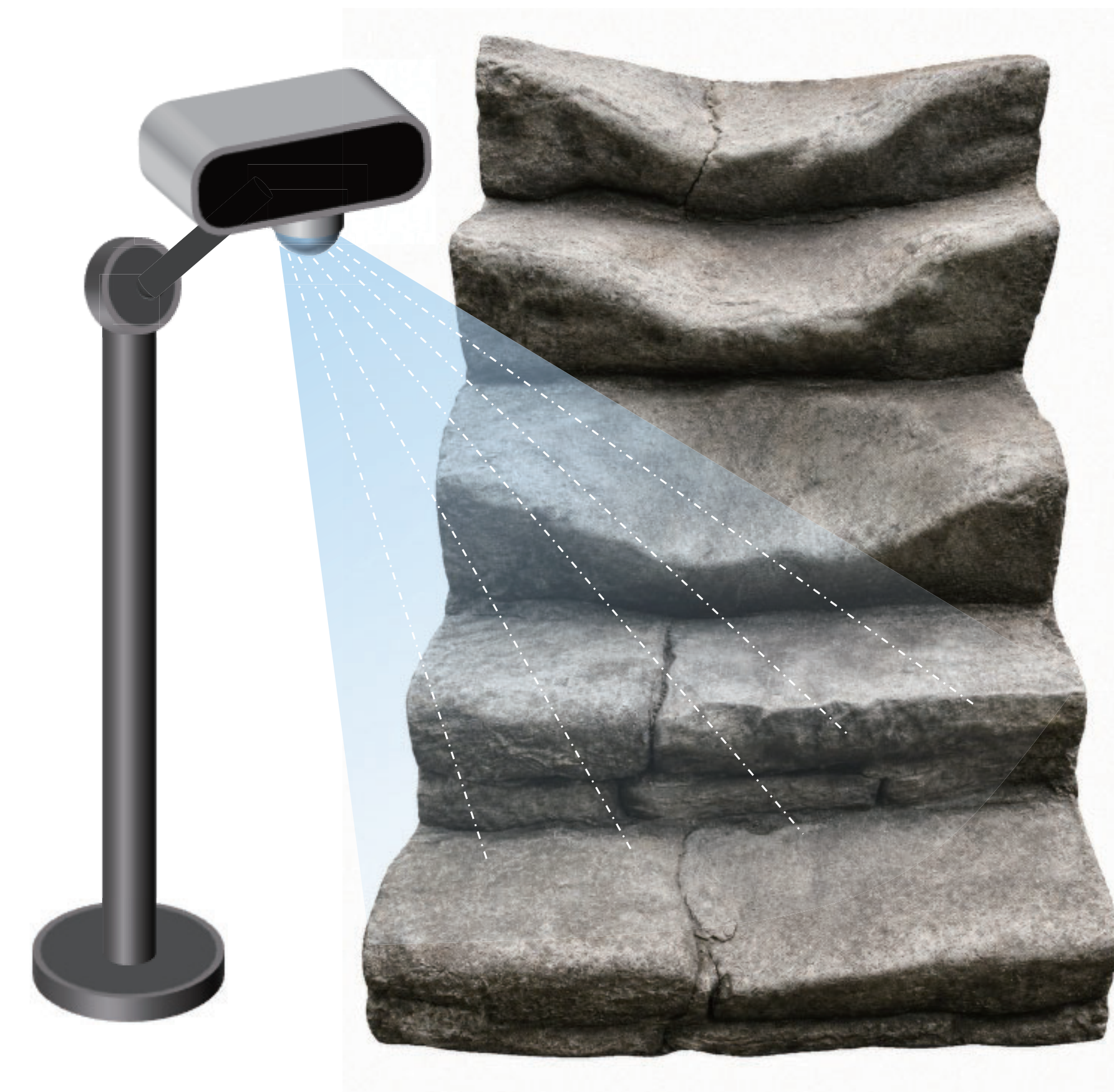
Intel RealSense D455 Non-contact 3D scanning of worn stone staircase
