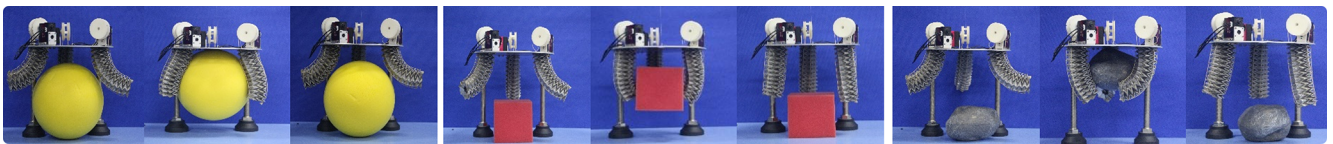
Figure 10. Grasping process diagrams of a sphere, a cylinder, and an irregular object.
