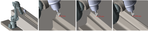
Figure 4. Robot end-effector in contact with segments A, B, and C of the switch rail.
