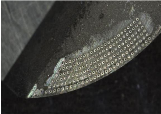
Figure 2. Tool-modified textured surface microstructure diagram.
