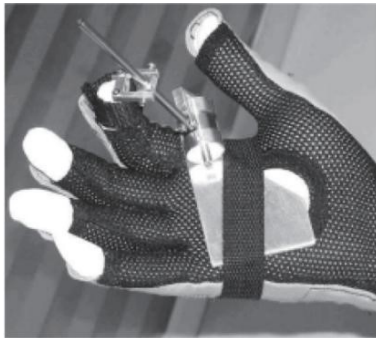
Figure 2. Magnetorheological fluid-based haptic actuator.
