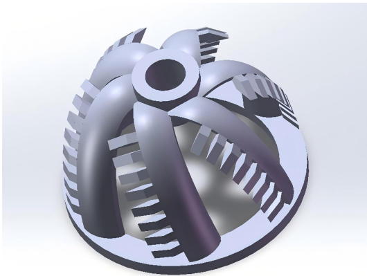
Figure 1. Three-dimensional model of the cutter head.
