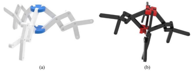
Figure 4. Angular-element groups. (a) Triangle-based mechanism with three angled elements. (b) Quadrangle-based mechanism with four angled elements.
