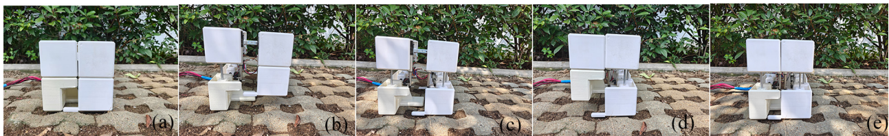
Figure 36. Linear locomotion of the HFCM in a rocky environment. (a) Initial state. (b) Foot1 lifts. (c) Foot1 falls. (d) Foot2 lifts. (e) Foot2 falls.
