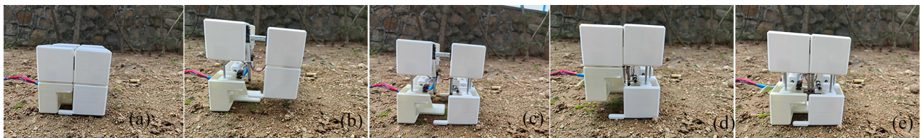
Figure 37. Linear locomotion of the HFCM in a sandy environment. (a) Initial state. (b) Foot1 lifts. (c) Foot1 falls. (d) Foot2 lifts. (e) Foot2 falls.
