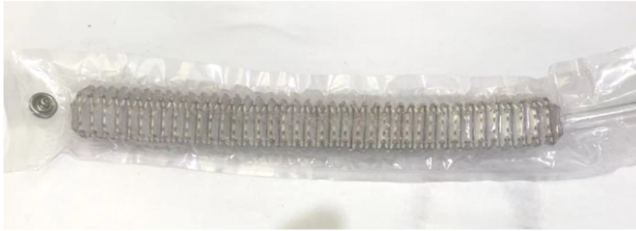
Figure 14. The prototype of the soft pneumatic actuator.
