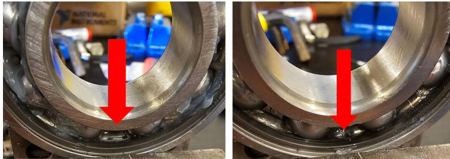
Figure 4. Outer race faults. Bearings with a damaged outer race: large fault – case 1 (left panel) and small fault – case 2 (right panel).
