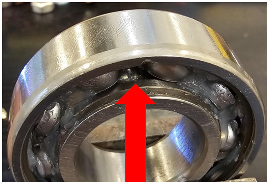
Figure 5. Bearing with damaged inner race.
