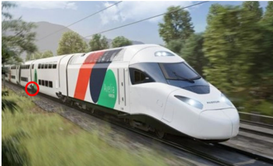
Figure 1. The Avelia Horizon. The position of damper bracket between the rear wall of the middle cars is circled (photo by Alstom).
