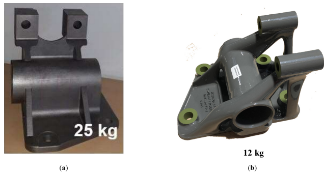
Figure 9. The damper bracket: (a) as conventional part, designed for casting or sheet metal welding; (b) as designed for the possibilities of additive manufacturing.
