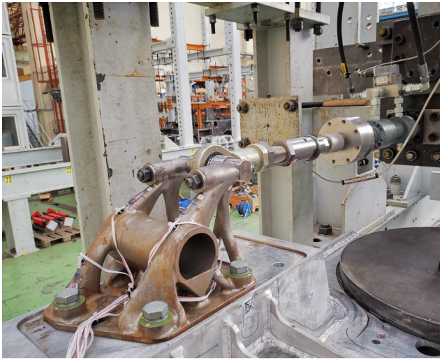
Figure 7. The damper bracket in the test rig.
