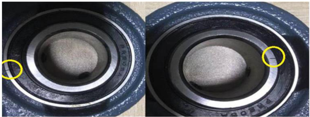
Figure 10. Inner- and outer-ring faults of the luffing mechanism bearing.
