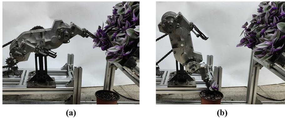
**Figure 18.** Photographs of seedling transplanting tests. **(a)** Seedling-pick-up operation. **(b)** Seedling-planting operation.
