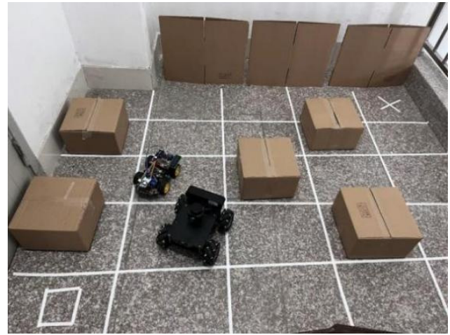
Figure 38. AGV is avoiding dynamic unknown obstacles.
