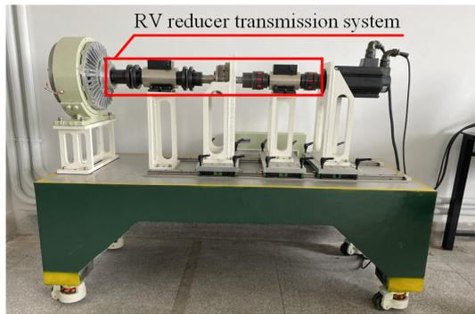
**Figure 1.** RV reducer performance parameter test device.
